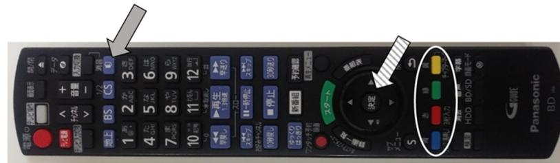
**Figure 2.** Television (TV) remote controller used in the Hybridcast TV system.
