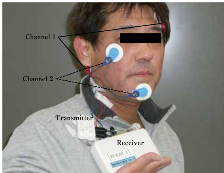
Figure1 The overview of 4 electrodes application and device including Transmitter and Receiver (ZA-9)
